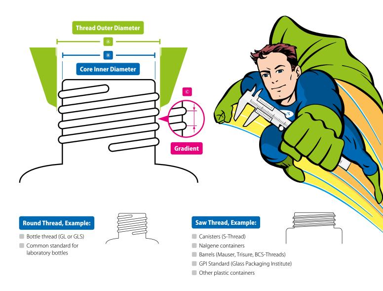
Note: All the measurements and values given here can vary up to 0.5 mm, dependent upon the manufacturer involved (due to manufacturing tolerances). Brand names and trademarks are the property of the respective owners. The brand names and protected trademarks mentioned here are simply of descriptional nature.
